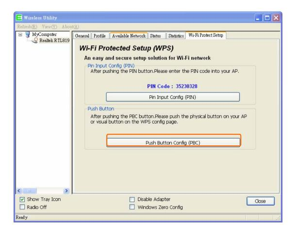
2. WU306n is waiting for the other AP to start the PBC function. The other AP starts the PBC function should be before WU306n WPS times out.
