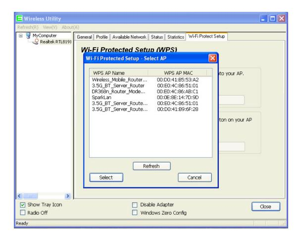
3. WU306n is waiting for the AP to establish the connection. And then enter the PIN code into the AP that you want to connect. For example, the AP uses BR360n to be the connecting device. Enter the PIN code into client pin number and then clicks the "Start PIN" button.
