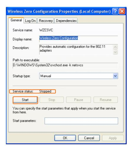
5. Once the setting completes, the "Service status" become to "Started". Click the "OK" button to finish it and the WU306n Wireless Utility can see the check option of "Windows Zero Config".
