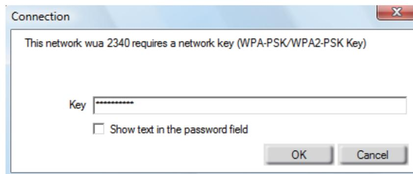
It is recommended to enable WPA-PSK on your wireless router or access point before configuring your wireless adapter. Make sure you enter the passphrase exactly the same on all wireless devices.
