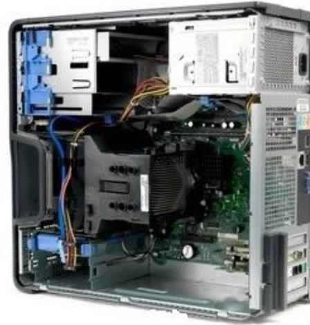
**Step 2:** Remove the metal cover bracket
