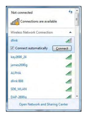
4. Enter the same security key or passphrase that is on your router and click **Connect**. You can also connect by pushing the WPS button on the router.
