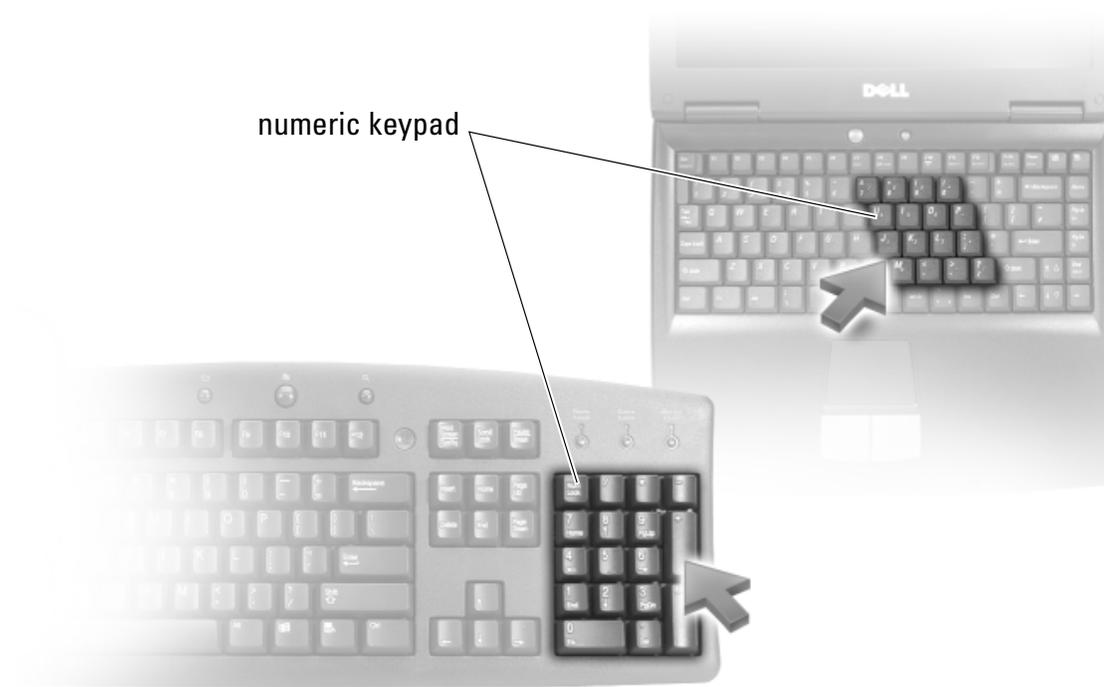
The numeric keypad functions like the numeric keypad on an external keyboard. Each key on the keypad has multiple functions. The keypad numbers and symbols are marked in blue on the right of the keypad keys. To type a number or symbol, hold down <Fn> and press the desired key.
