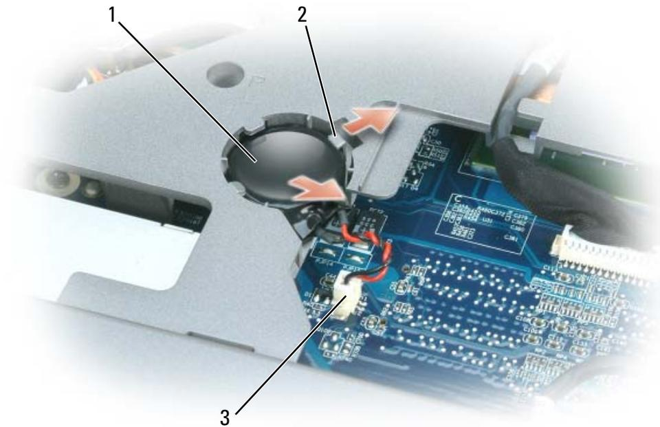
1 coin-cell battery      2 release latch      3 battery cable connector
