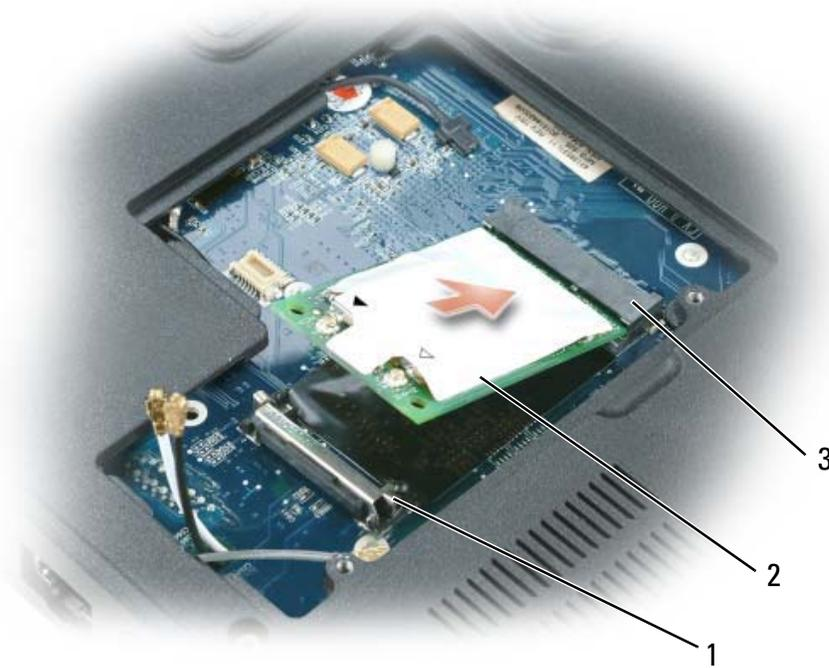
1 securing clips    2 antenna connectors (2)    3 Mini-Card connector
