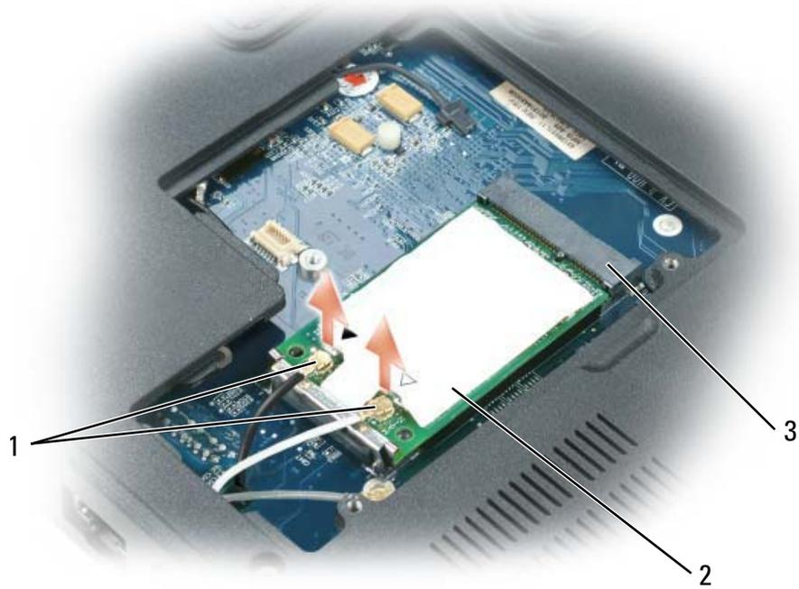
1 antenna cables (2)      2 Mini-Card      3 Mini-Card connector
