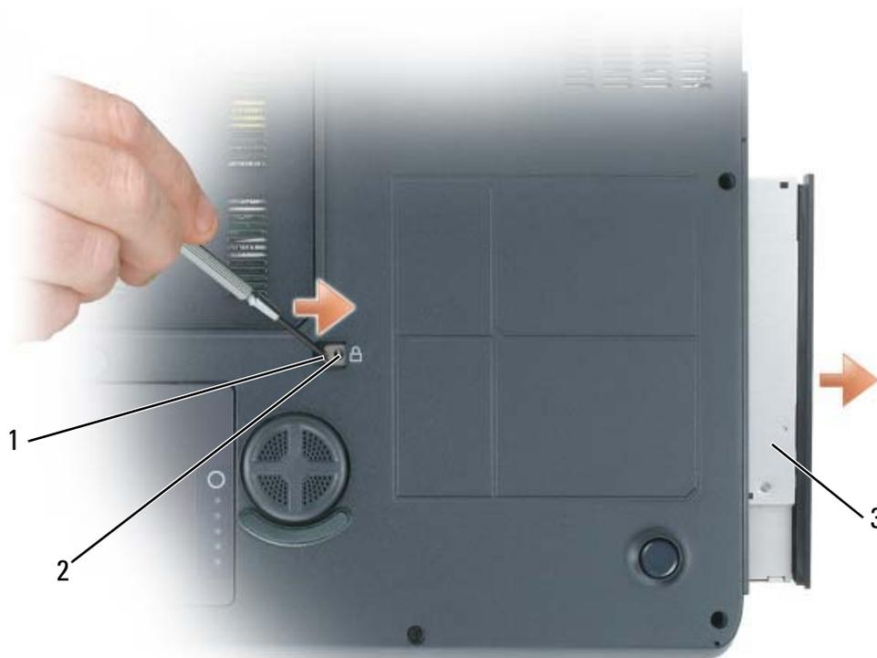
1 notch                      2 optical-drive security screw    3 optical drive
