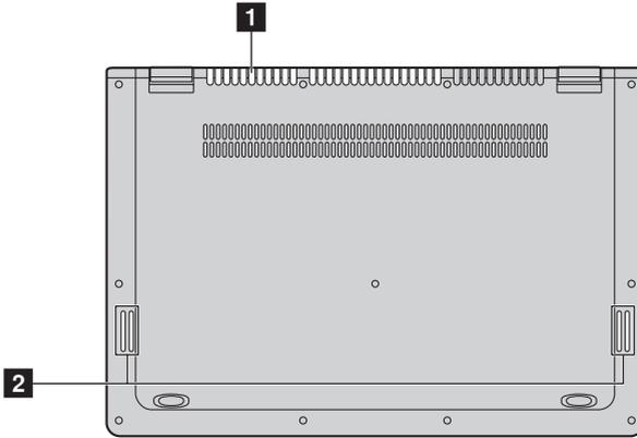
**1 Ventilation slots** Allow air to enter the computer for cooling.
