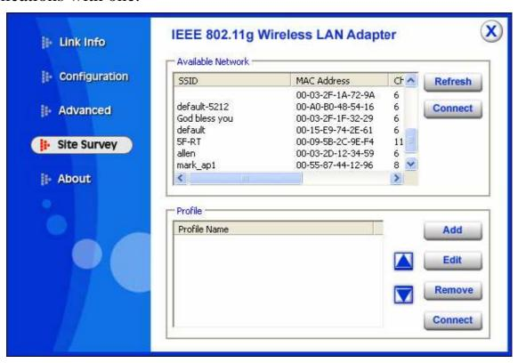
**Available Network** – displays the wireless networks (wireless clients and Access Points) that are in signal range.
