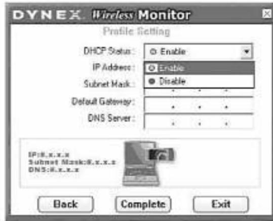
The purpose of this screen is to configure the TCP/IP setting of each wireless connection. You must define if the current profile's IP setting is assigned by a DHCP server or assigned by a fixed IP that is determined by the Network Administrator.
