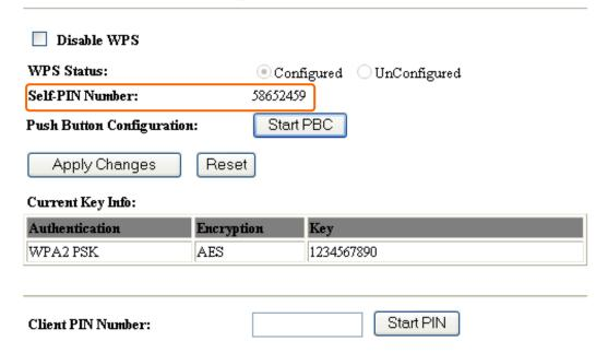
3. Enter the PIN Code that from the enrollee AP into the "Pin Code" text. Click the "PIN" button to start the PIN of WPS function.
