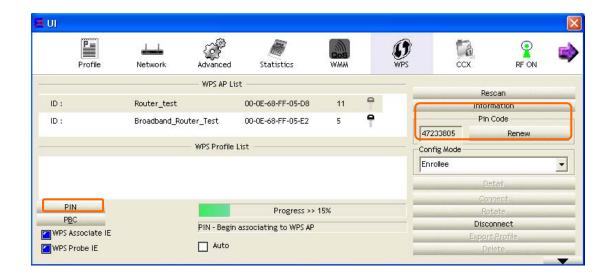
3. Enter the PIN code into registrar AP. For example, the AP uses BR360n to be the connecting device. Enter the PIN code into client pin number and then clicks the "Start PIN" button.
