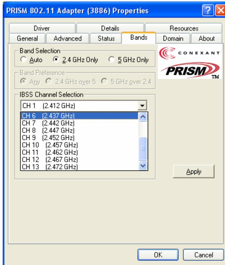
**Figure 5.4** Band Tab for 2.4 GHz only
