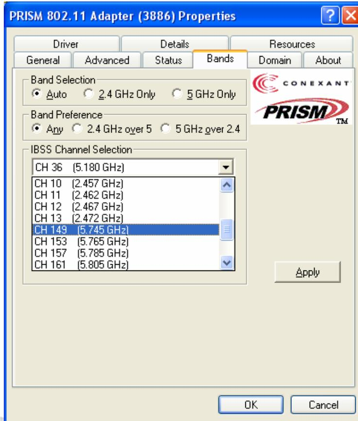
**Figure 5.3** Band Tab for Auto selection (2.4 or 5Ghz)
