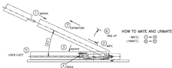
**Figure 1.1:** Insertion and Removal of the Mini-PCI Board
