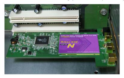
2. Install all three antennas on the wireless network card, and make sure the antennas are securely installed. To improve radio reception, please adjust antennas to the position shown in the left picture.
