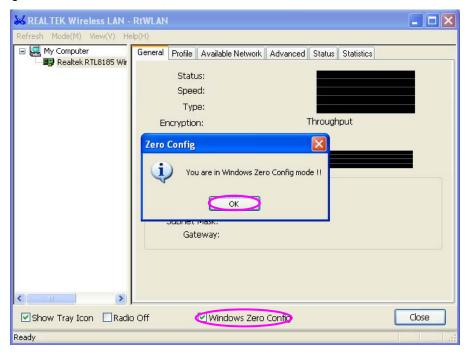
C. Uncheck "Windows Zero Config" to enable the utility of the adapter.
