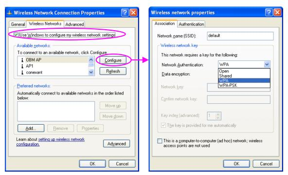
3. Press "Configure" button to configure the WPA function for the current network.
