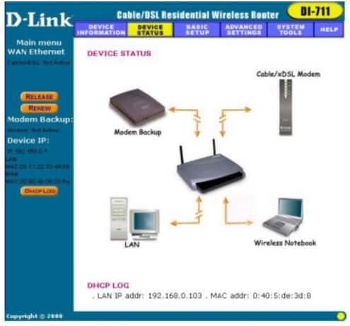
The Device Status screen displays a graphical representation of your current configuration. The left side of the screen shows your connection information in regards to WAN and LAN IP Address information. The right side displays the connection status of each device.
