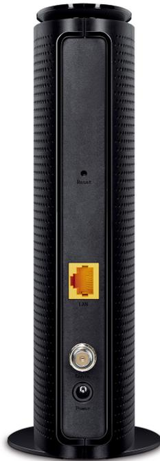
The back panel provides the Reset button and several connection ports. Refer to the following for detailed instructions.
