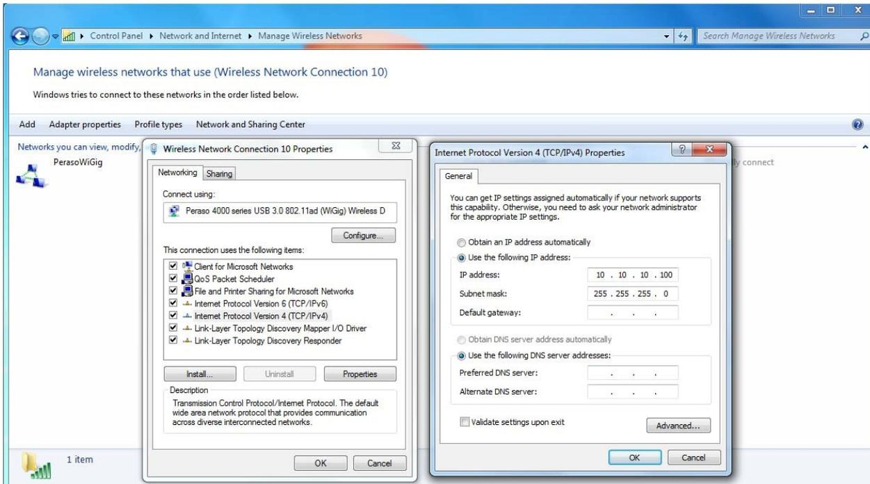
Figure 3-2-6: Configuring static IP addresses
