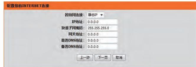
The screenshot shows the 'Configure your INTERNET connection' window. The 'Internet connection' dropdown is set to 'Static IP'. Below it are input fields for 'IP address', 'Default subnet mask', 'Gateway address', 'Preferred DNS address', and 'Alternate DNS address'. At the bottom are three buttons: 'Previous Step', 'Next Page', and 'Cancel'.
