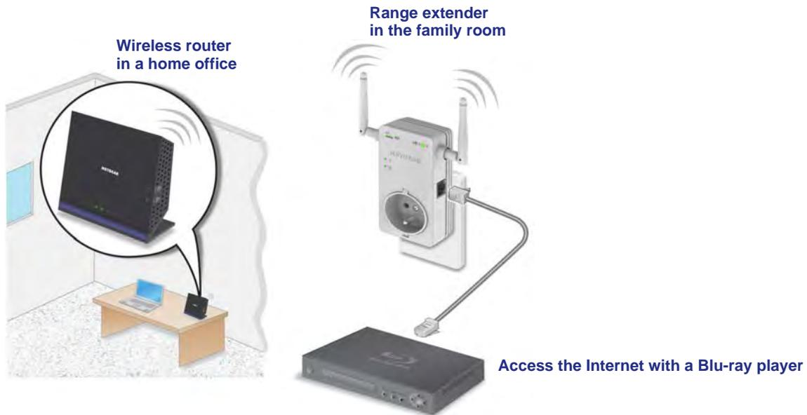
Figure 5. Extender Ethernet port connection
