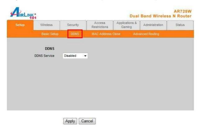
To Enable DDNS, select the DDNS provider you have registered with and enter the required fields. Click **Apply** to save the setting.
