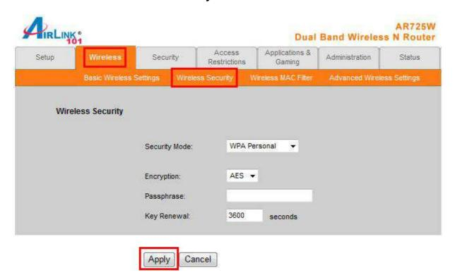
**Encryption**: Select either **TKIP** or **AES** or **AES** as the encryption method.
