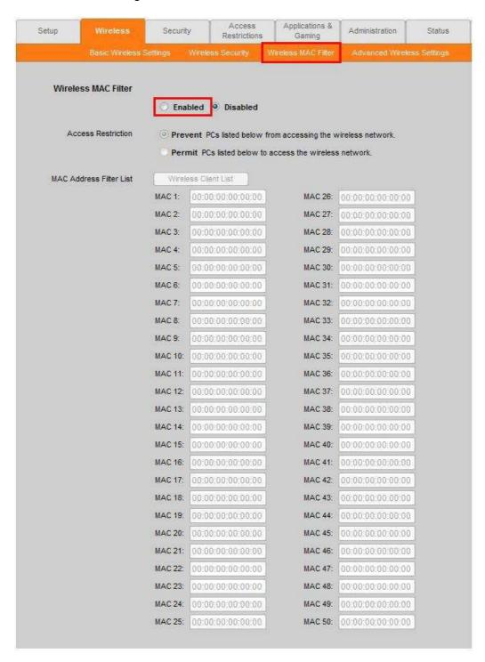
Select **Enabled** and choose whether the specified wireless clients will be prevented or permitted to access the wireless network. Enter their MAC address in the fields below and click **Apply** to save the setting.
