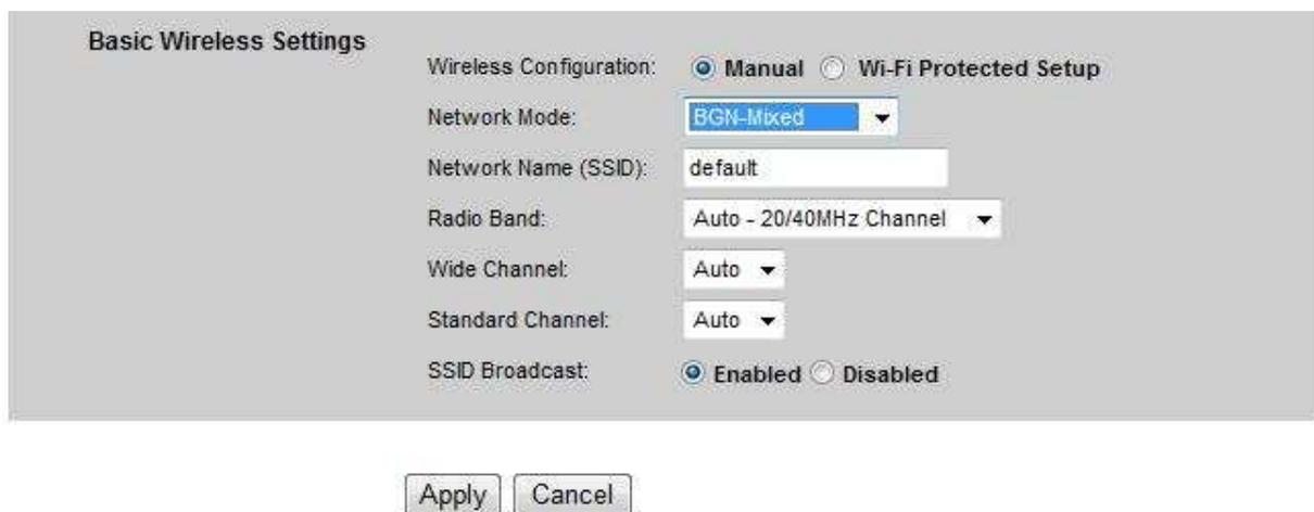
**Network Mode:** If you have 802.11b/g/n 2.4GHz devices on the wireless network, select **BGN-Mixed**. If you have 802.11a/n 5GHz devices on the wireless network, select **AN-Mixed**.
