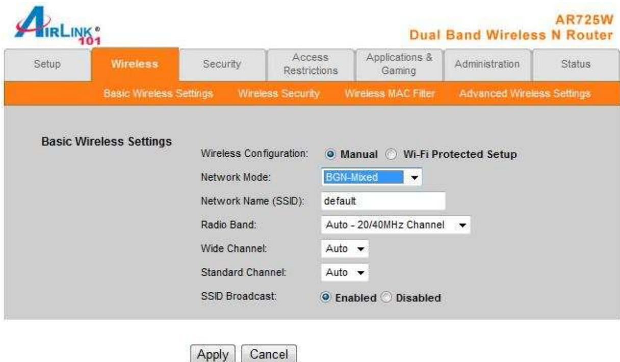
The screenshot shows the web interface of the AIRLINK 101 AR725W Dual Band Wireless N Router. The top navigation bar includes tabs for Setup, **Wireless**, Security, Access Restrictions, Applications & Gaming, Administration, and Status. Below this, there are sub-tabs for Basic Wireless Settings, Wireless Security, Wireless MAC Filter, and Advanced Wireless Settings. The main content area is titled "Basic Wireless Settings" and contains the following configuration options:
