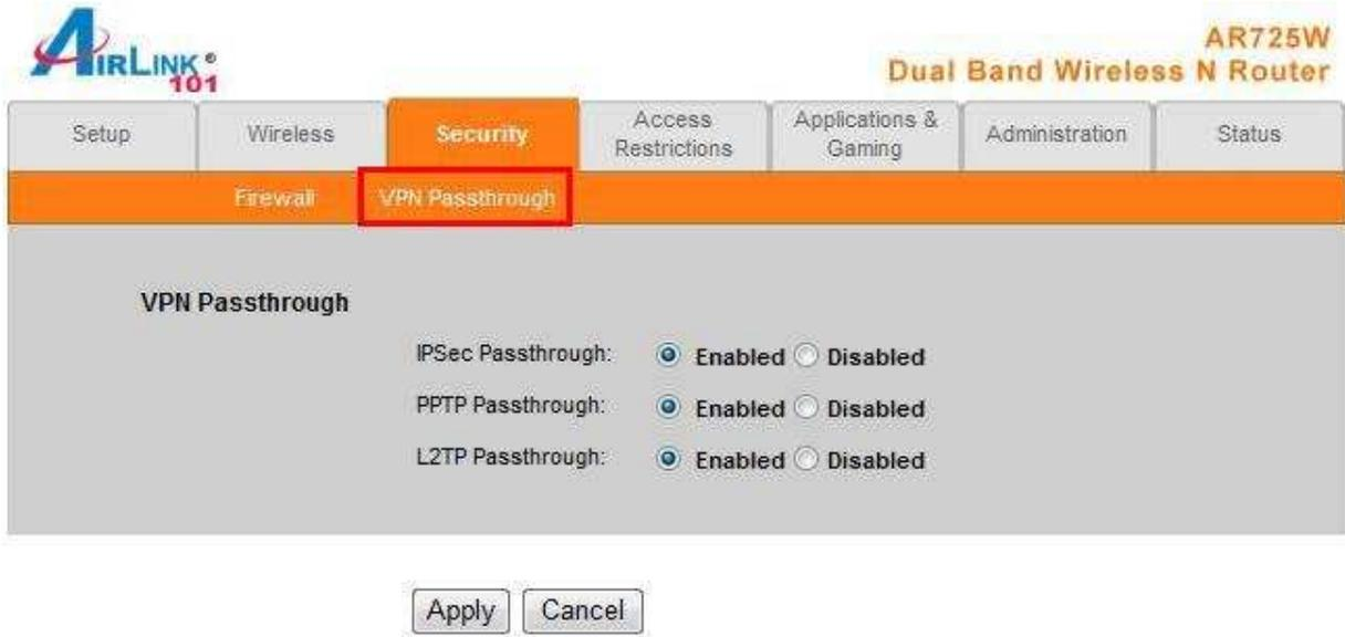
The screenshot shows the configuration interface for an AirLink 101 AR725W Dual Band Wireless N Router. The top navigation bar includes tabs for Setup, Wireless, Security, Access Restrictions, Applications & Gaming, Administration, and Status. The Security tab is selected, and the VPN Passthrough sub-tab is highlighted with a red box. Below the navigation bar, the VPN Passthrough settings are displayed:
