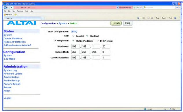
Figure 13 Static IP under switch mode
