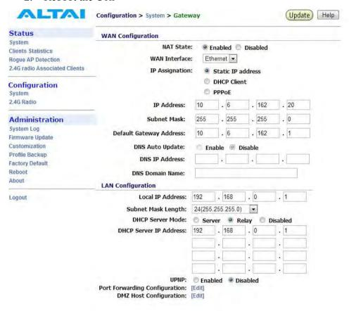
Figure 17 Configure DHCP Relay Server
