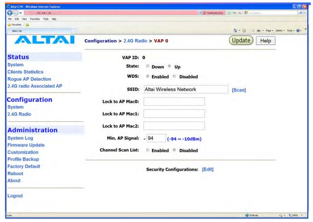
Figure 23 Station Mode Configuration
