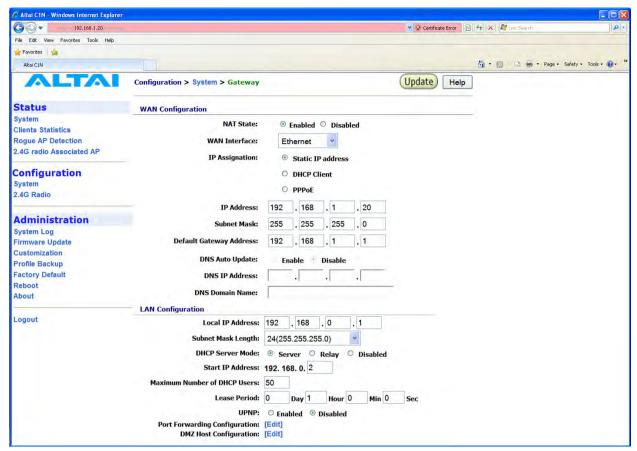
Figure 14 Network Configurations under Gateway mode
