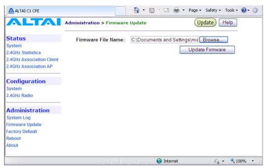
Figure 43 Upload the Firmware through HTTP
