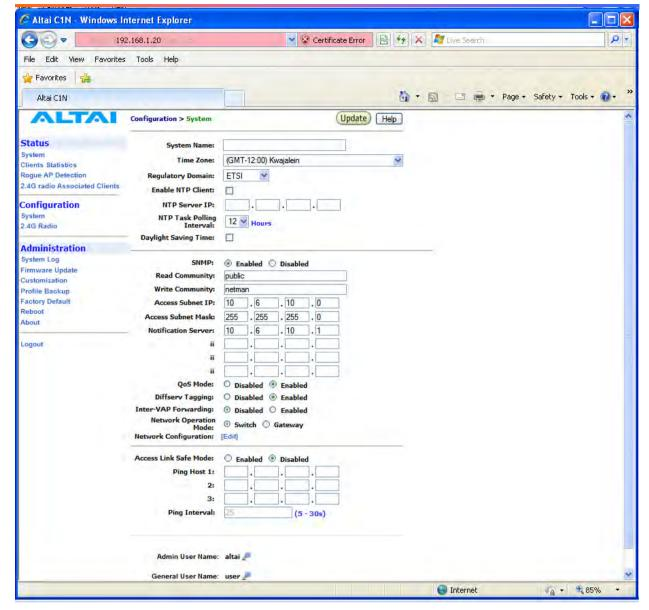
Figure 10 SNMP Configuration
