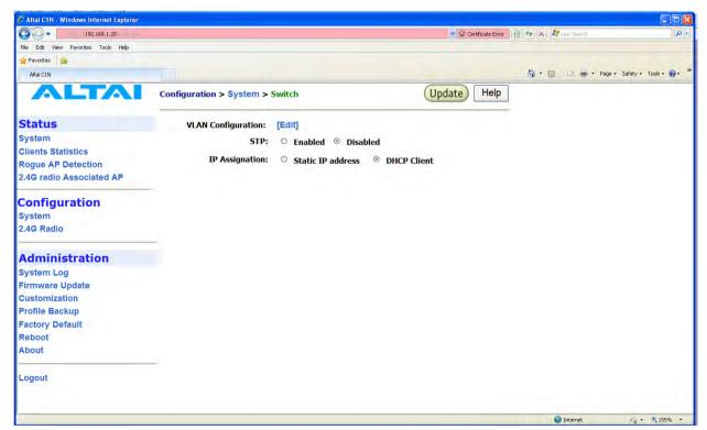
Figure 12 DHCP client under Switch mode
