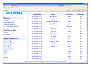
Figure 24 2.4G Radio Channel Scanning
