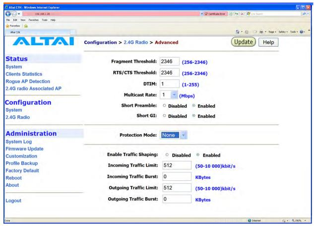
Figure 22 Bandwidth Control Configuration
