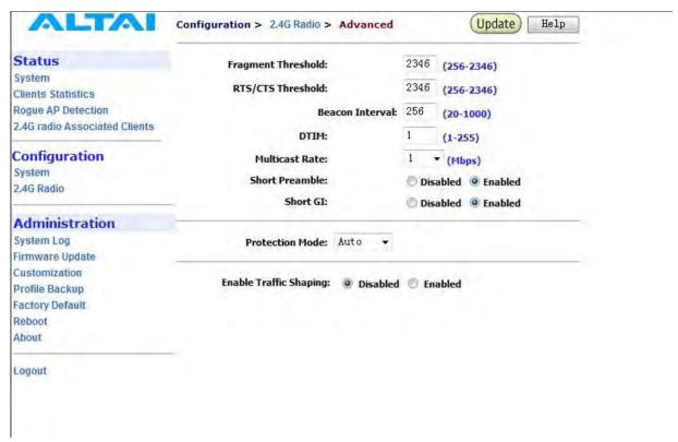
Figure 21 Advanced 2.4GHz Radio Setting
