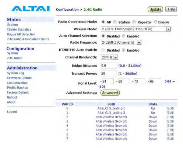
Figure 20 2.4GHz Radio Parameter Configuration
