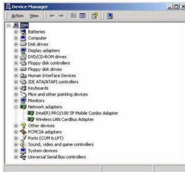
If there is Question-mark (?) or Exclamation-mark (!) in yellow on your WLAN CardBus Adapter in previous picture (PC Card Properties & System Properties), please make sure you have inserted the right PC Card, the proper driver and utility have been installed as well. If you are not sure, follow the procedure below to reinstall (update) the driver.
