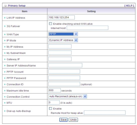
1. LAN IP Address: The local IP address of this device. The computer on your network must
