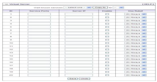
For example, if you have an FTP server (port 21) at 192.168.123.1, a Web server (port 80) at 192.168.123.2, and a VPN server at 192.168.123.6, then you need to specify the following virtual server mapping table:
