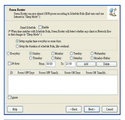
Step 6-2: Click SMART Schedule setting for Green function. The device would check the packet flow before the power is turned off. For instance, if the router is on the sleeping mode, you could surf the Internet at that time. Afterwards, if there are not any packet flows, the router would be
