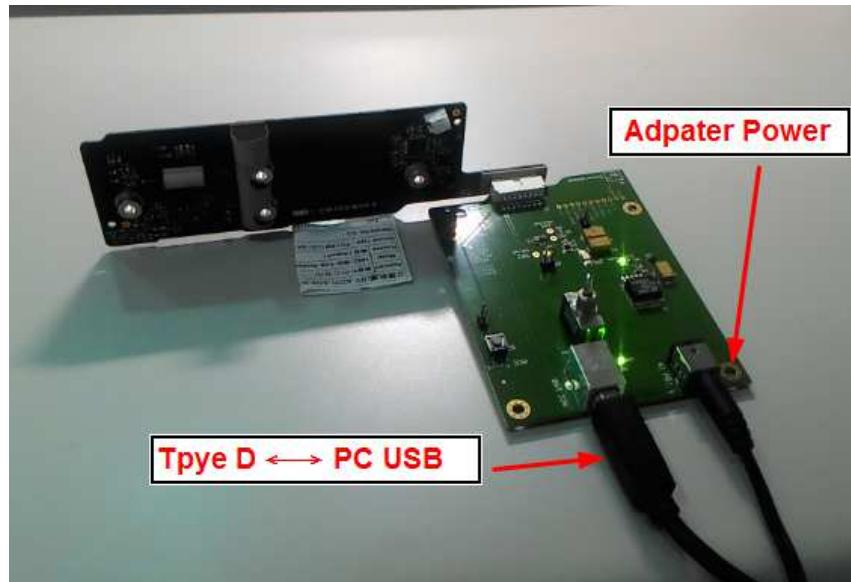
Step1. Insert Type D to PC USB & Adapter , Find new device and install driver as below path .
