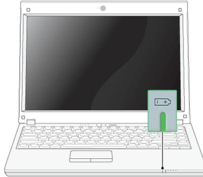
4. To remove the battery pack, push the Lock button to the direction of Unlock and lift the battery pack in the direction of the arrow.
