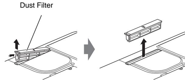
Figure 48. Removing the dust filter
