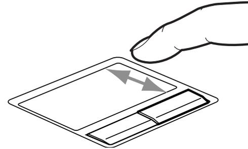
Figure 23. Scrolling with the Scroll Strip
