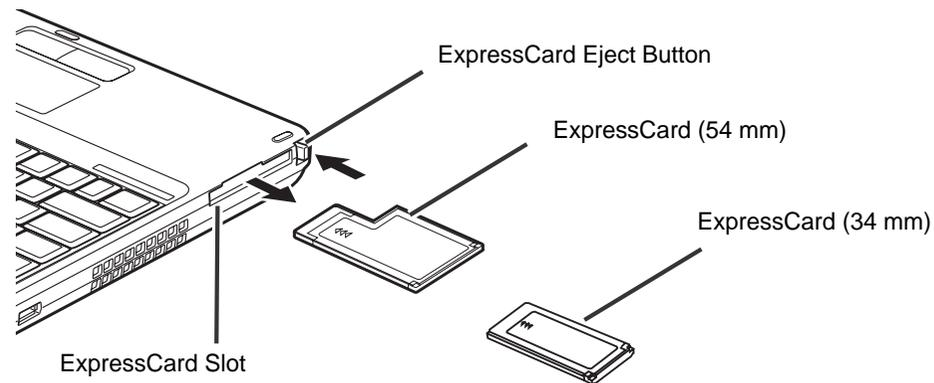
**Figure 37. Installing/Removing an ExpressCard**
