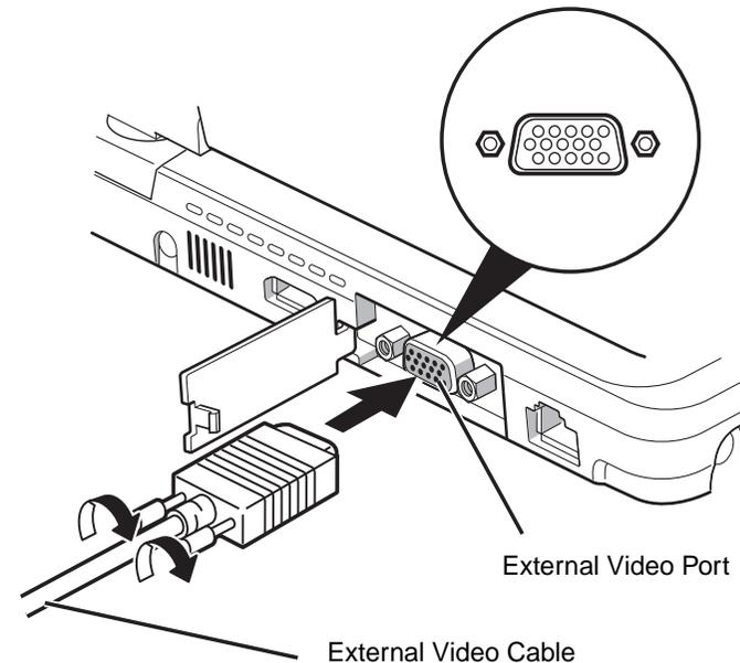
**Figure 47. Connecting an External Video Device**
