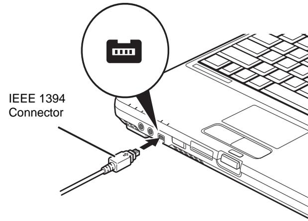
Figure 45. Connecting an IEEE1394 Device
