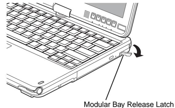
Figure 31. Removing/Installing Modular Bay Device
