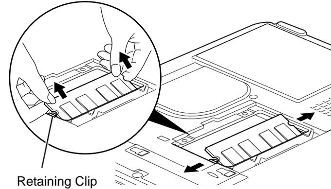
**Figure 39. Installing a Second Memory Module**
