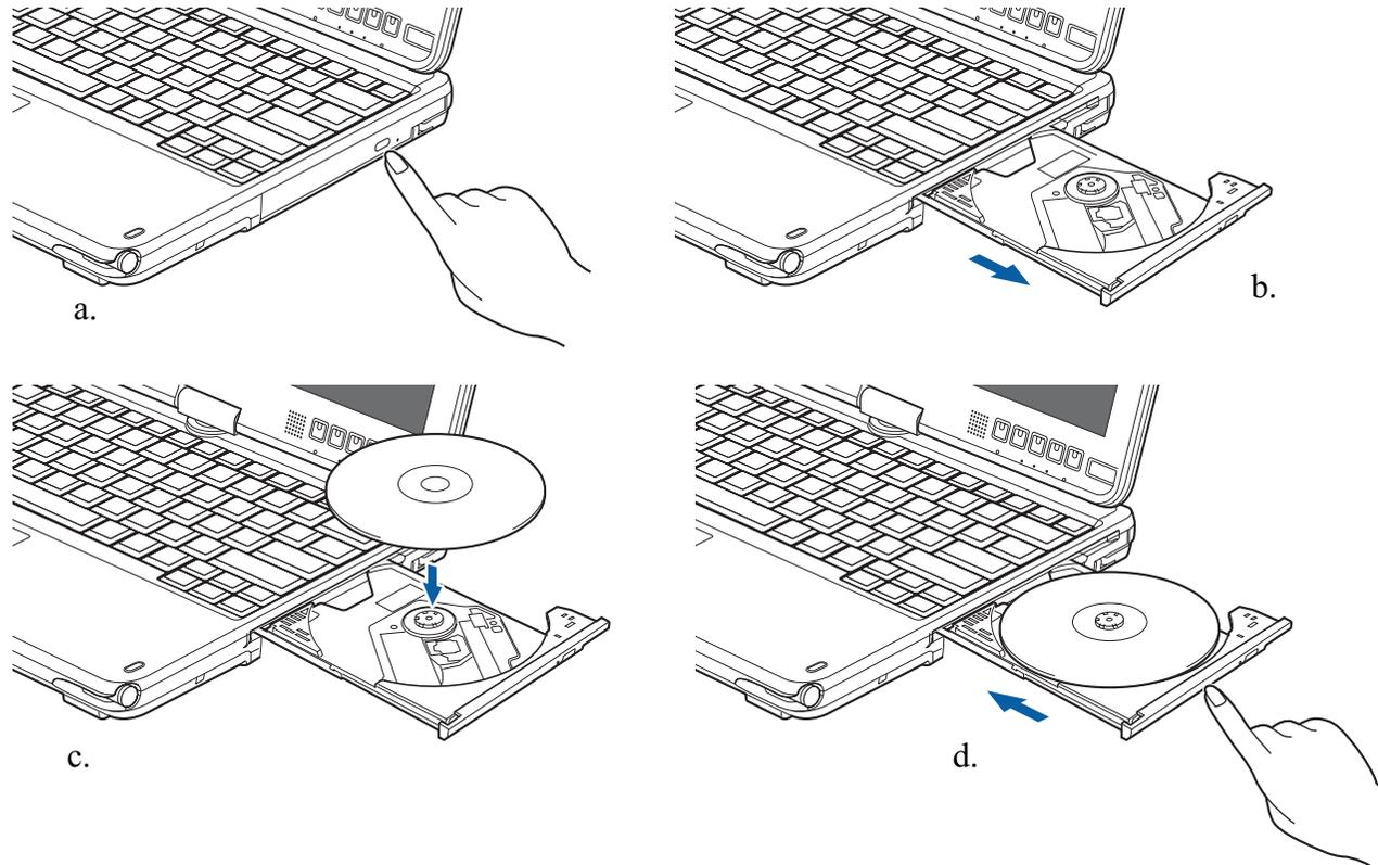
Figure 41. Loading/Ejecting Media
