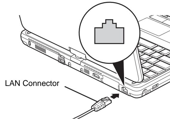
Figure 43. Connecting the LAN
