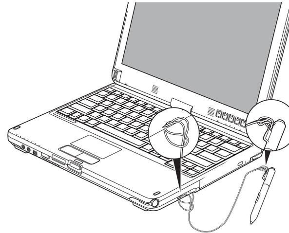
**Figure 29. Installing a Pen Tether**
