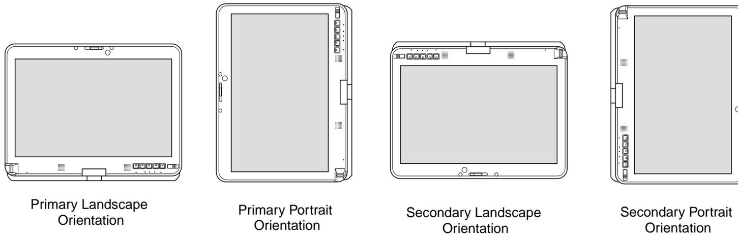
**Figure 13. Orientations for Tablet PC in Tablet Mode**
