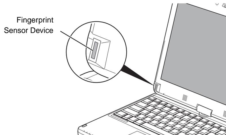
**Figure 52. Fingerprint sensor**
