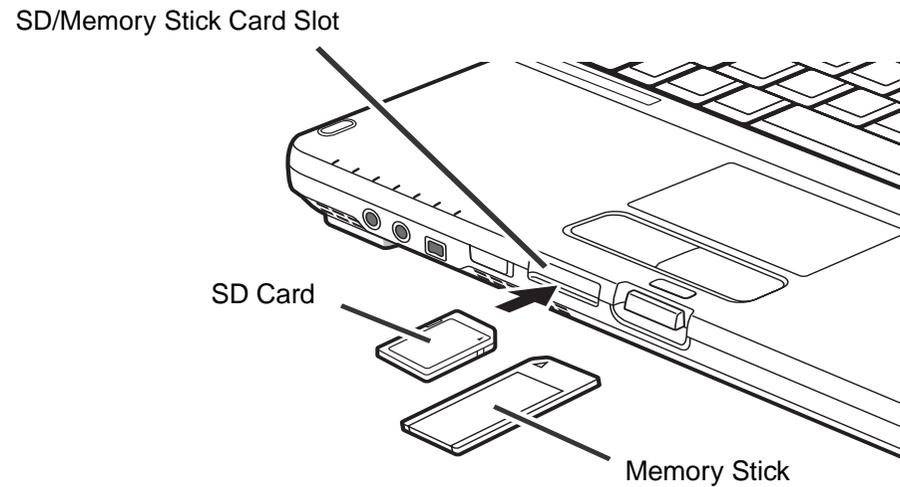
**Figure 36. Installing a Memory Stick or SD Card**
