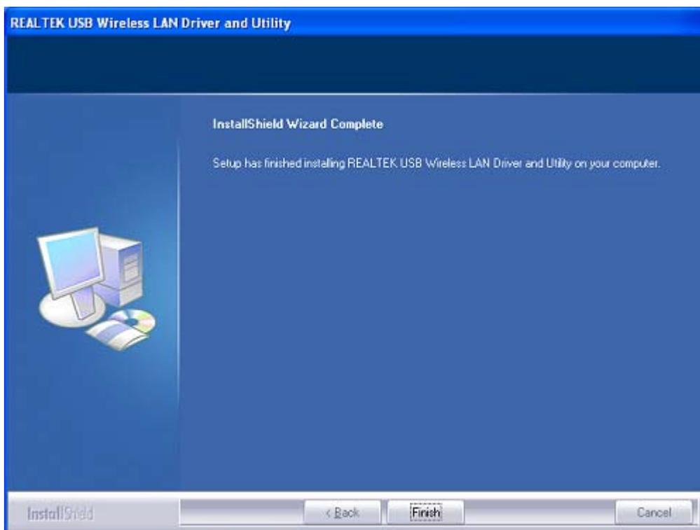
8. After click **Finish** to complete the installation , under Windows XP <ALL Programs> menu , REALTEK USB wireless LAN Utility program installed.
