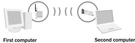
You can use the same adapter to join different wireless networks (and different types of wireless networks) at different times. For example, you might use your adapter to connect to an infrastructure network at home most of the time, but occasionally, you might use your adapter to set up a temporary ad hoc network to share files with a colleague who visits you at your home office.
