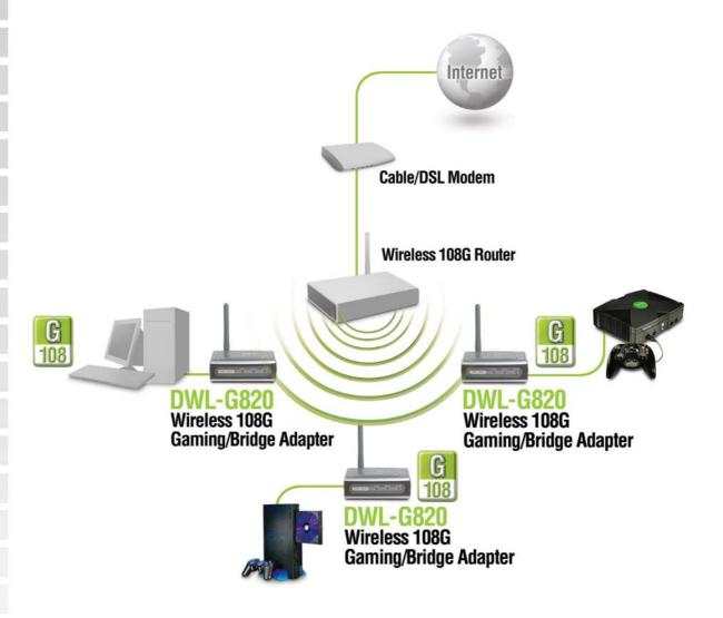
This example illustrates an **Infrastructure** setup. To connect the DWL-G820 to a wireless network with a wireless router or access point, please refer to the printed Quick Installation Guide included with the product. Web configuration is required to connect the DWL-G820.
