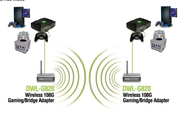
This example illustrates an **Ad-Hoc** setup. Simply connect the DWL-G820 (*refer to the Quick Installation Guide*) to your Ethernet-capable network device *(in this case, a gaming console*) and you will be able to connect wirelessly with other gaming consoles also connected to DWL-G820s.
