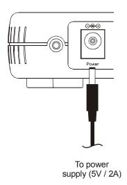
2 Plug the power adapter into a grounded and surge protected power outlet. The Power LED on the front panel lights green when connected properly.
