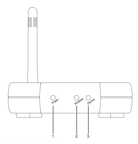
The LEDs of the unit indicate its operational status.
