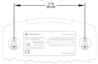
The illustration is drawn at a one-to-one scale, which means that when printed, it provides the exact dimensions required to mount the unit.
