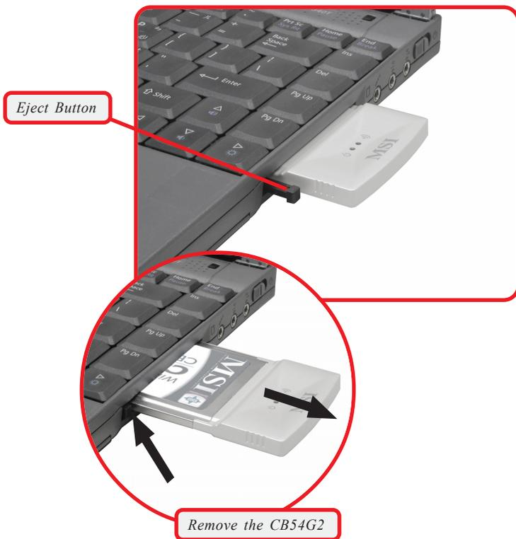
*Before removing the CB54G2, you should stop the device in Windows operating system.*
