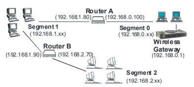
Figure 38: Routing Example
