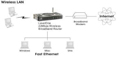
Figure 1: LevelOne 22Mbps Wireless AP Router
