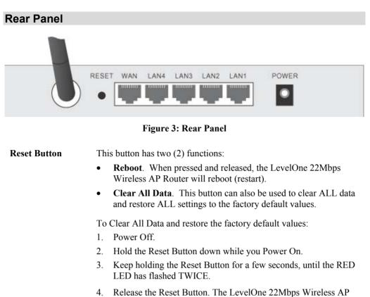
Router is now using the factory default values.WAN portConnect the DSL or Cable Modem here. If your modem came with a
