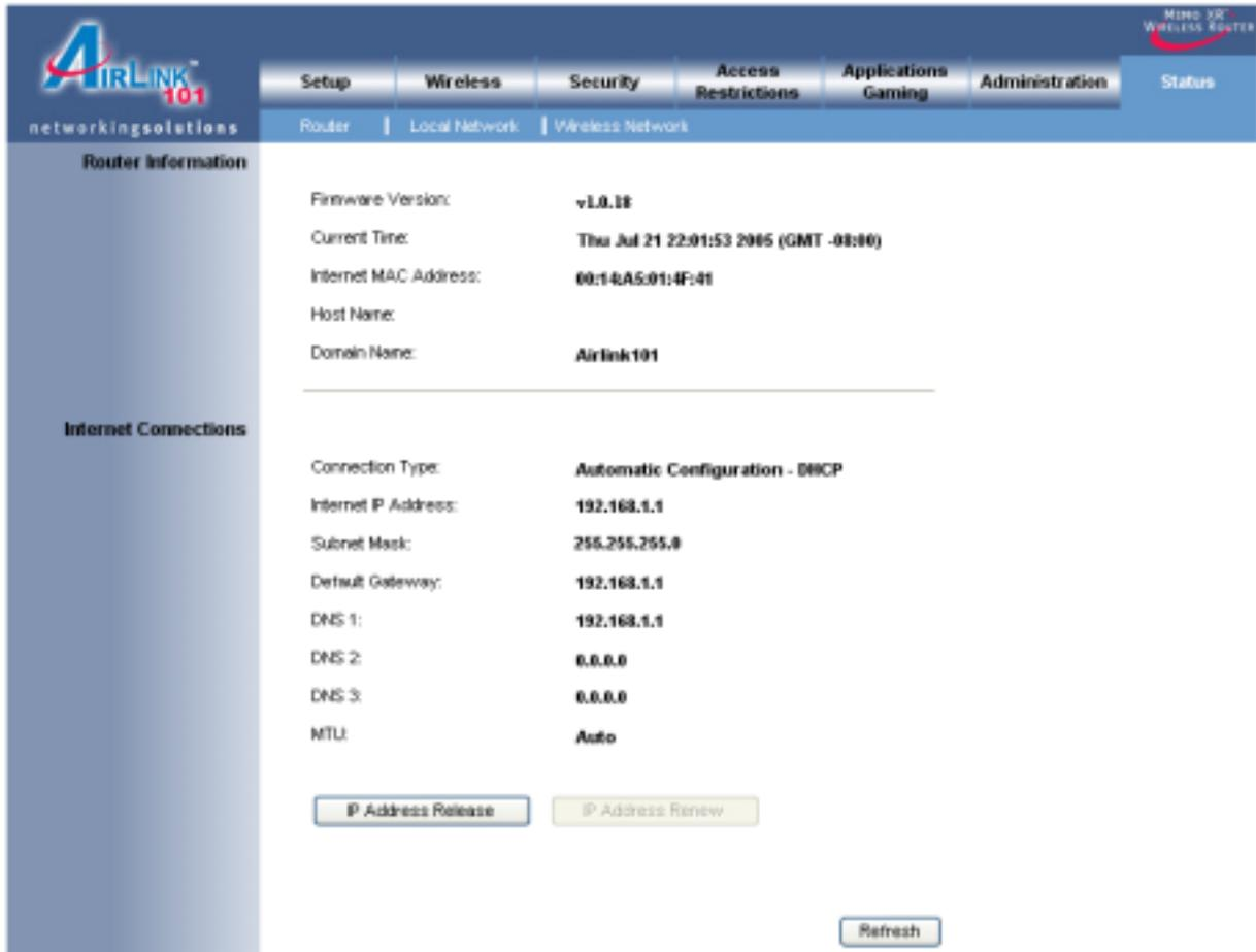
The screenshot displays the web interface of an Airlink 101 router. The top navigation bar includes tabs for Setup, Wireless, Security, Access Restrictions, Applications Gaming, Administration, and Status. The Status tab is active, showing Router Information and Internet Connections.
