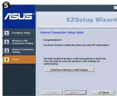
Setup is complete, press **Print/Save Wireless LAN Settings** button for future reference. Click **Finish** to exit the EZSetup utility.
