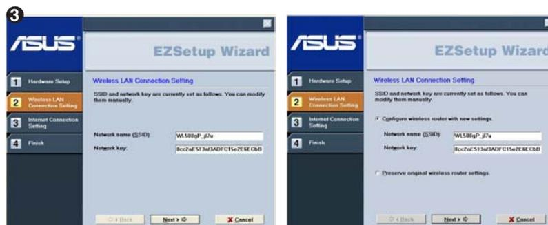
Wireless settings, including network name and network keys, are generated automatically. You can modify these settings manually. Note if your wireless router is configured before, select **Preserve original wireless router settings** to use the current value. Click **Next** to continue.
