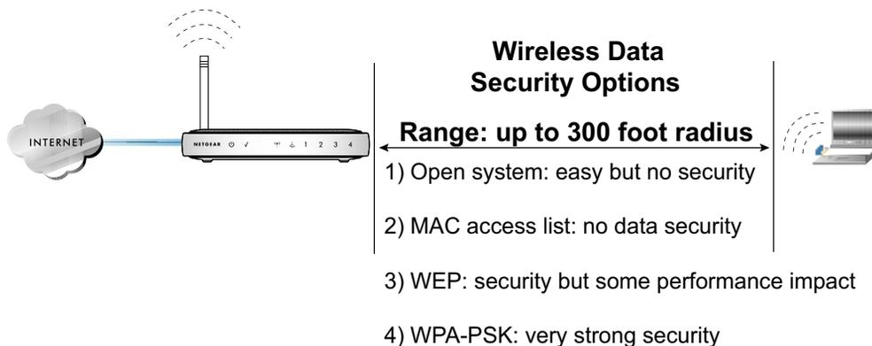
**Figure 4-1: wireless router wireless data security options**
