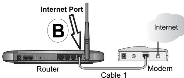
**Figure 3-2: Connect the wireless router to the modem**
