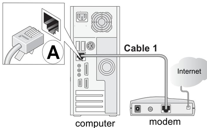
**Figure 3-1: Disconnect the Ethernet cable from the computer**
