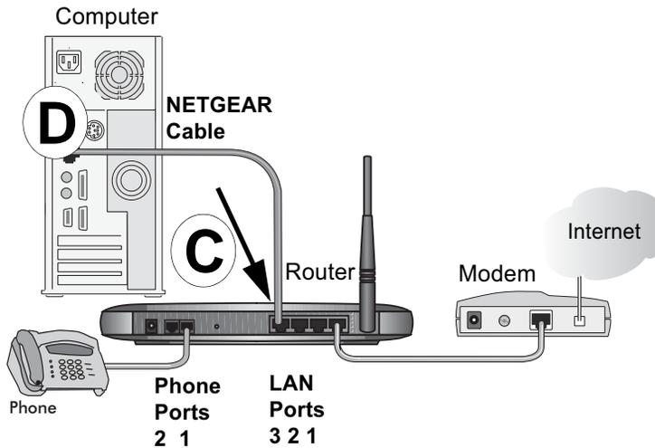
**Figure 3-3: Connect the computer to the wireless router**
