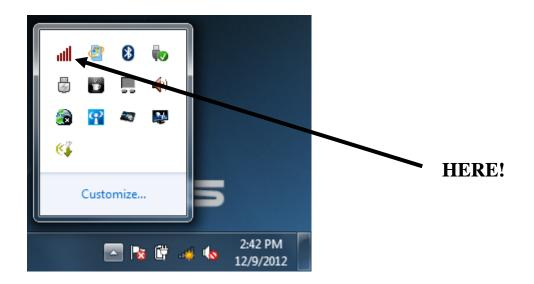
Left-click the icon will launch wireless network configuration utility, and you can right-click the icon to show the quick menu of configuration utility. This icon also uses different color to show the status of wireless connection:
