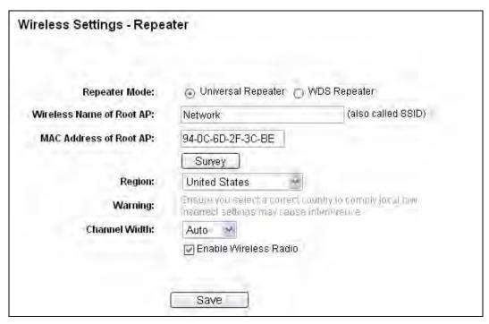
Figure 4-12 Wireless Settings in Repeater mode
