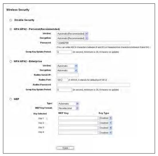
Figure 4-15 Wireless Security - Access Point
