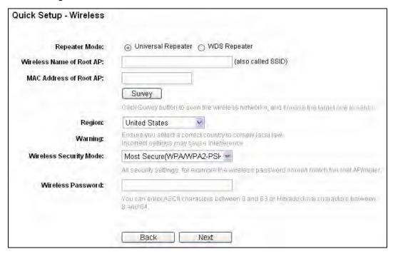
Figure 3-13 Wireless Settings - Repeater(Range Extender) mode
