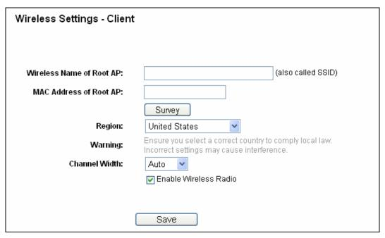
Figure 4-14 Wireless Settings in Client mode
