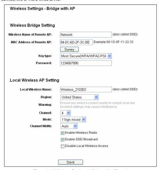
Figure 4-13 Wireless Settings in Bridge with AP mode
