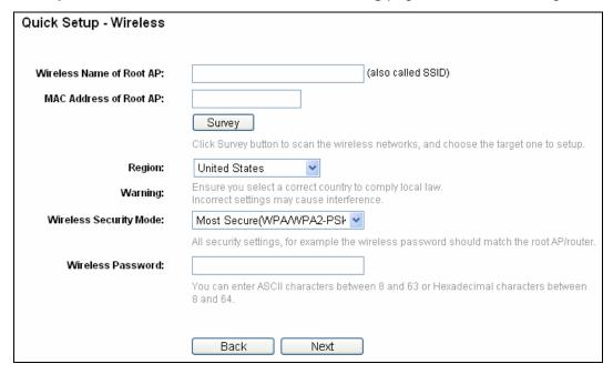
Figure 3-17 Wireless Settings - Client mode
