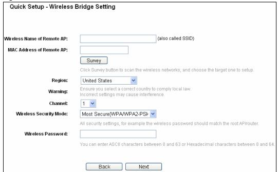
Figure 3-15 Wireless Settings – Bridge with AP mode
