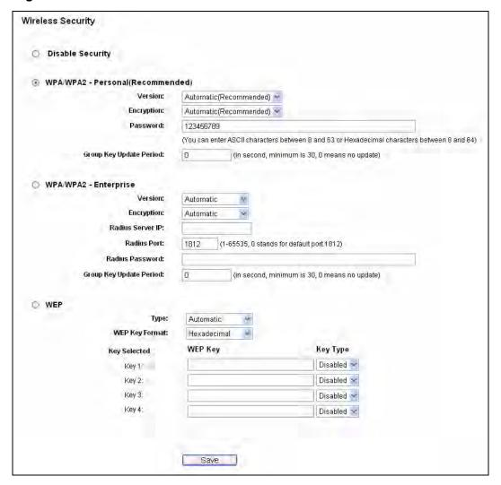
Figure 4-18 Wireless Security – Bridge with AP
