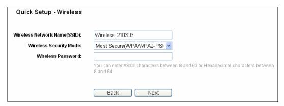
Figure 3-11 Wireless Settings - Access Point mode
