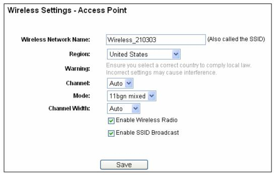
Figure 4-10 Wireless Settings in Access Point mode
