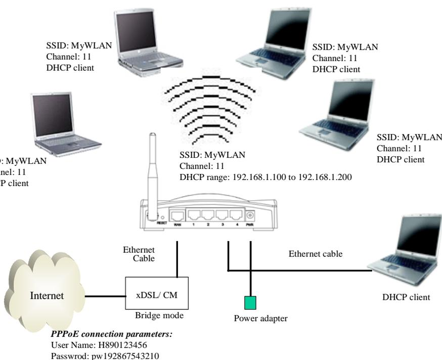
Figure 3 – Configuration Example One – PPPoE on the WAN
