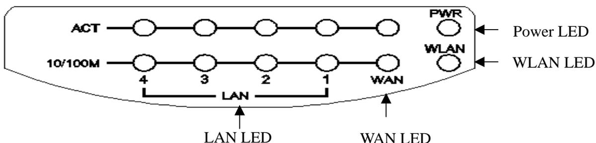
Figure 1 –WLAN 11G AP ROUTER Front Panel
