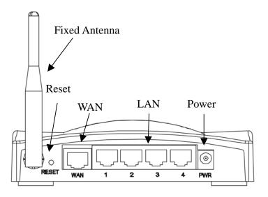
Figure 2 – WLAN 11G AP ROUTER Rear Panel (Fixed Antenna)
