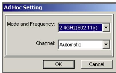
4. In the **Start Ad Hoc** drop-down list, select the wireless standard (802.11b or 802.11g) for your Ad Hoc computer-to-computer network.
