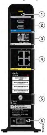
**Important:** Do not connect your PC to both the Ethernet and USB ports at the same time. Your residential gateway will not function properly if both the Ethernet and USB ports are connected to your PC at the same time.
