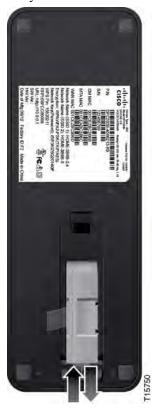
5 Close the battery compartment door. The battery lock will automatically reengage.
