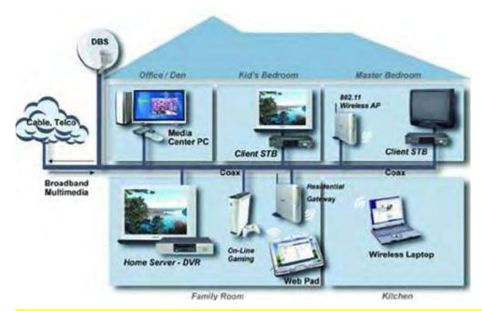
MoCA operates over the physical layer of the home coaxial cable plant in the 1000-1500MHz spectrum. Its infrastructure begins at the service provider's drop cable at the first passive splitter connected to the home coax network.
