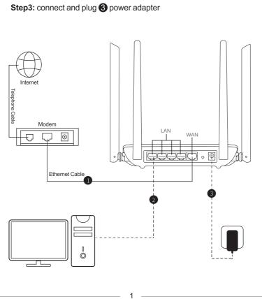
Step1: connect modem to router via 1 Wan port by ethernet cable
