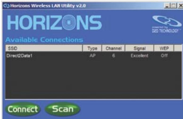
The top-most section of the D2D Configuration Dialog Box shows the available connections. The available connections will be displayed from a scan performed when the software was started, or when the scan button was clicked.
