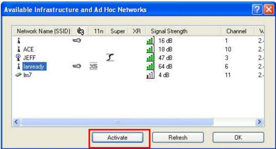
Step 2 Verify that the adapter has adequate Signal Strength.
