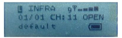
In "lock mode" the detector constantly refreshes the signal strength so the user can move around to find where the detected signal strength is the strongest.
