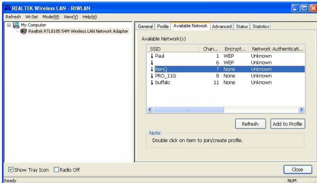
If you want to add one Access Point to the profile, click “**Add to Profile**” button. The [Wireless network properties](#) windows will display. You can configure your Wireless Network Security for the card.
