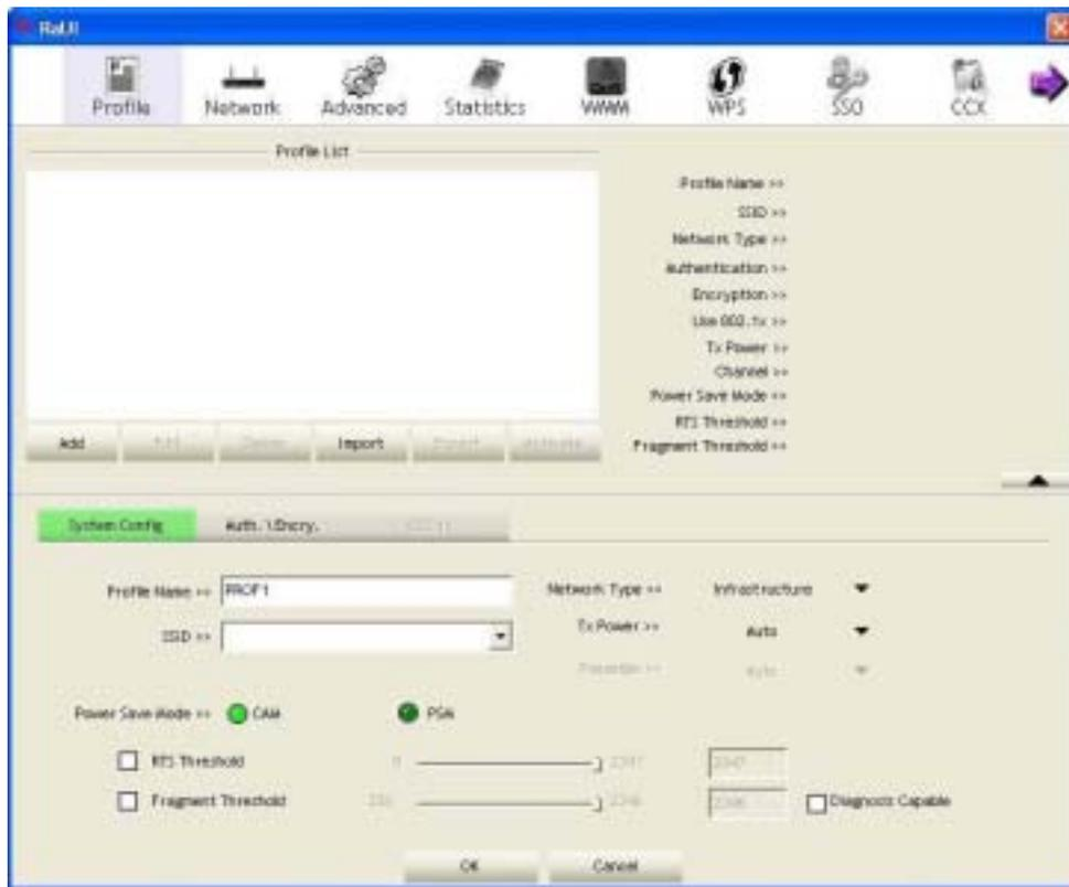
**Step 3:** Change profile name to what you want to connect. Pull down the SSID and select one intended AP. The AP list is the result of last Network.
