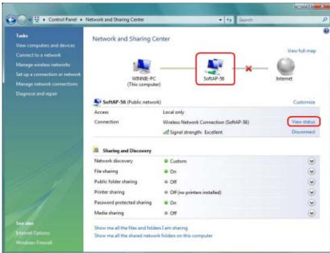
**Step 10:** In General tab, click "Detail...", and then you can see the current Network connection details. If this computer is successful connect to SoftAP-56 Access Point, the DHCP server will be assigned to same IP address.
