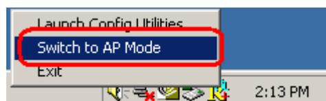
**Step 6:** After switch to AP mode, Ralink Wireless Utility will automatically pup-up. The Wireless Default SSID is assigned as "SoftAP-56".
