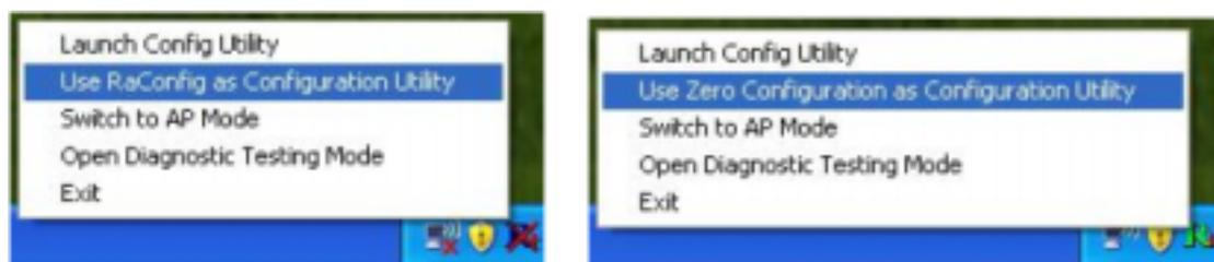
If “Use Zero Configurations as Configuration utility” is selected, please continue on the section. Below picture shows that the RaUI status when WZC is active as main control utility.
