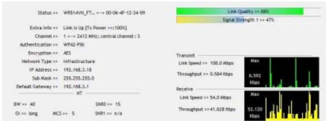
**Status:** Current connection status. If no connection, it will show Disconnected. Otherwise, the SSID and BSSID will show here.
