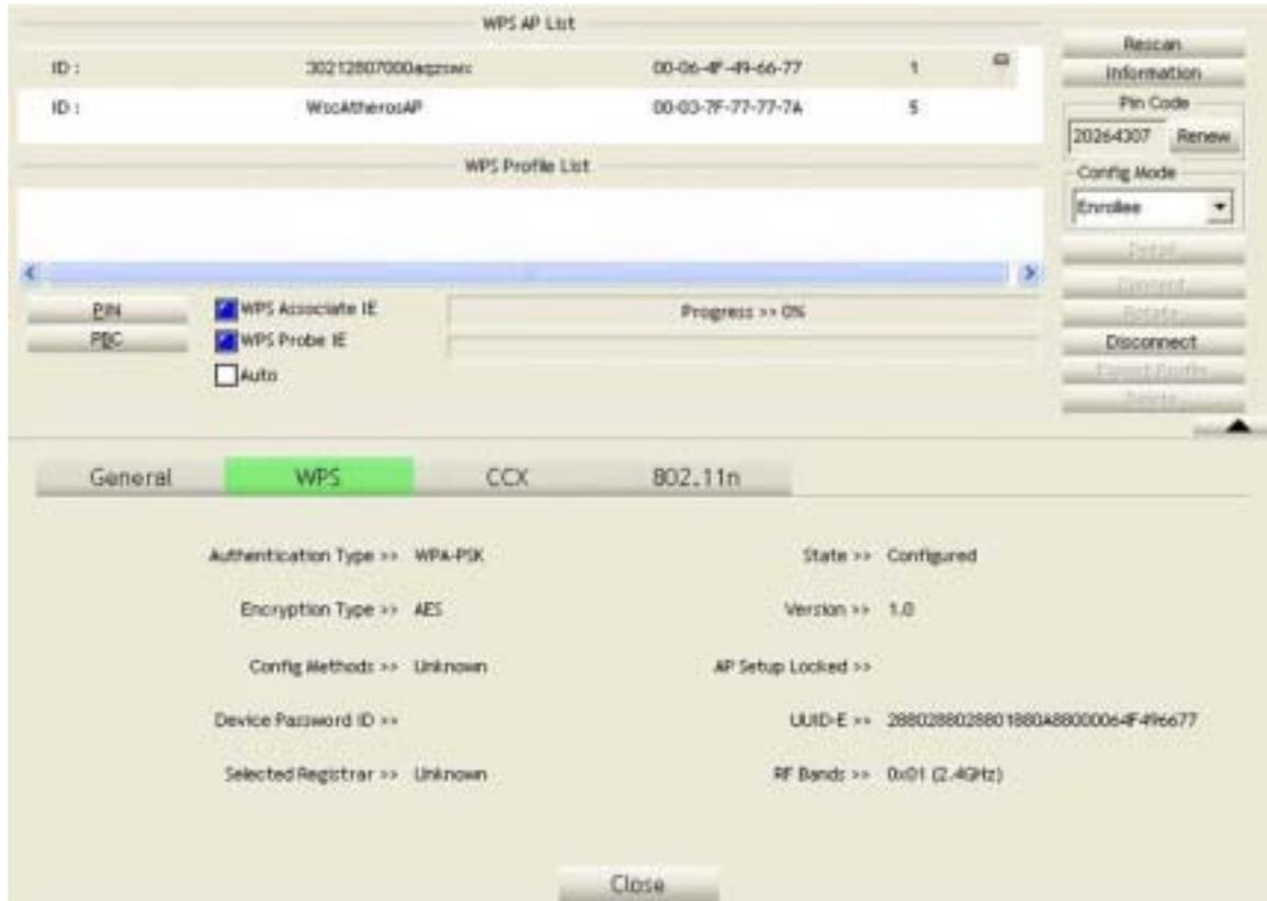
**Config Methods:** Correspond to the methods the AP supports as an Enrollee for adding external Registrars. (A bitwise OR of values)
