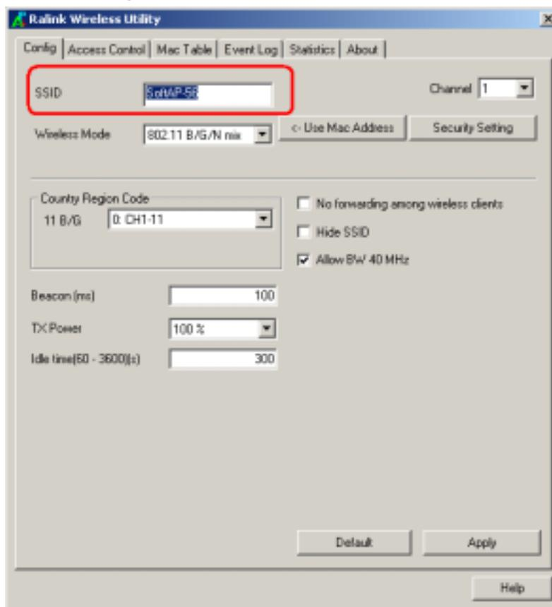
**Step 7:** To make sure your Soft AP is working properly, you need to use another computer which with Wireless LAN feature to access SoftAP-56 AP. In the below example, use another PC with Wireless feature in Vista Operation System. Go to **Start → Control Panel → Choose "Network and Sharing Center"** option → Click "Connect to a network" to search the available networks.
