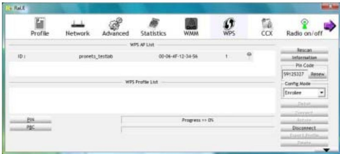
**WPS Configuration:** The primary goal of Wi-Fi Protected Setup (Wi-Fi Simple Configuration) is to simply the security setup and management of Wi-Fi networks. Ralink STA as an Enrollee or external Registrar supports the configuration setup using PIN configuration method or PBC configuration setup using PIN configuration method or PBC configuration method through an internal or external Registrar.
