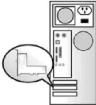
**STEP3:** Secure this card to the rear of the computer chassis and put back the cover.
