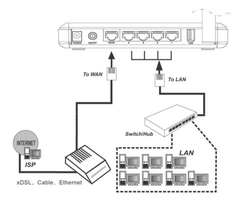
Figure 2-1 Hardware Installation of the PW-RN401/PW-RN401D 150Mbps Wireless Lite-N Router
