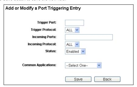
Figure 4-35 Add or Modify a Port Triggering Entry
