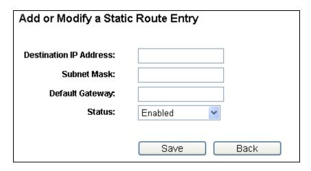
Figure 4-58 Add or Modify a Static Route Entry
