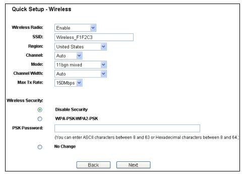
Figure 3-9 Quick Setup – Wireless
