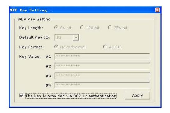
The key is provided via IEEE 802.1X authentication: Place a check in this box is IEEE 802.1X authentication is used. By selecting this option, the WEP key settings will be disabled.
