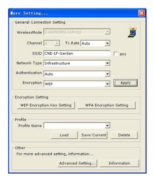
**SSID:** Enter the SSID of the network. The SSID is a unique name shared among all points in your wireless network. The SSID must be identical for all points in the network, and is case-sensitive. Place a check in the **any** box if you would like the device to connect to the first available Access Point with the strongest signal.
