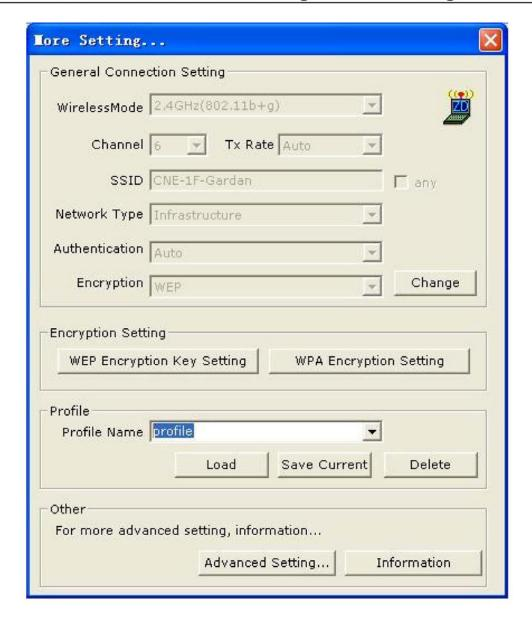
**Profile Name:** Displays the name of current profile. One device can have many profiles, but only one profile can be loaded at a time.
