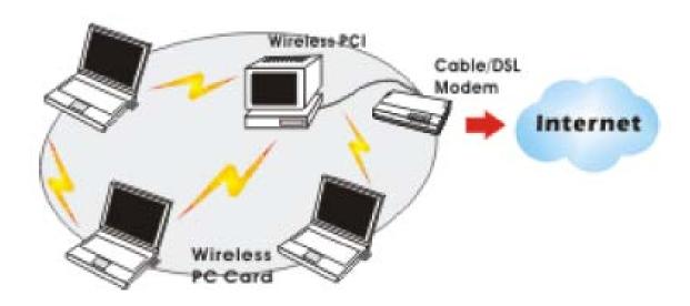
The Access Point Network The network installation allows you to share files, printers, and Internet access much more conveniently. With Wireless LAN Cards, you can connect wireless LAN to a wired global network via an Access Point.
