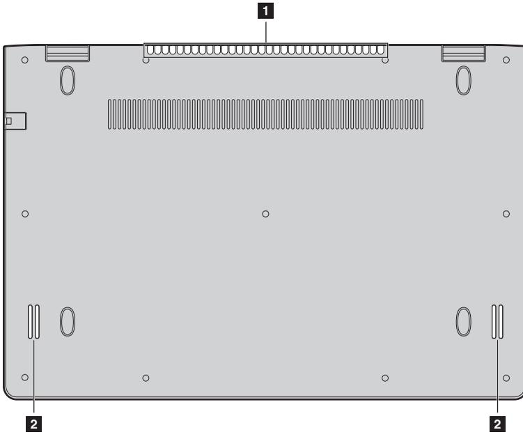
**1 Ventilation slots** Dissipate internal heat.
